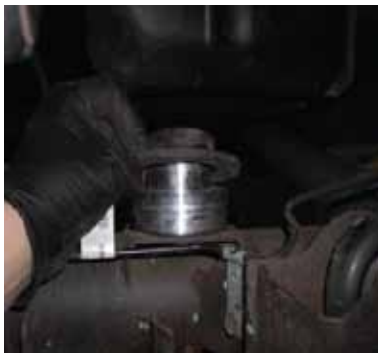
8. Use a jack to support the axle, this will allow you to lower and raise the axle as you need during installation. Unbolt the lower sway bar end link on both sides with a 17mm wrench.
