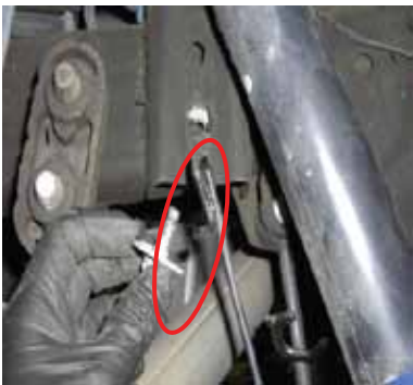
4. Using a 13mm socket, remove the brake line support bracket bolt.
