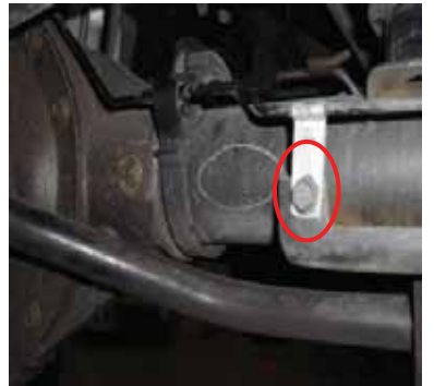
3. For vehicles with Autoride use a flat screw driver and pry the linkage off the upper trailing arm.
