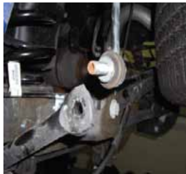
5. Remove the hard brake line support bracket bolt located next to the lower track bar mount on the driver side.
