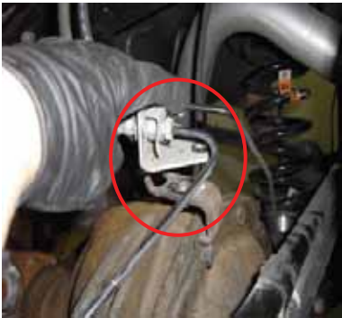
1. Remove the rear wheels. Unhook the ABS line located at the upper trailing arm mount on both sides.
