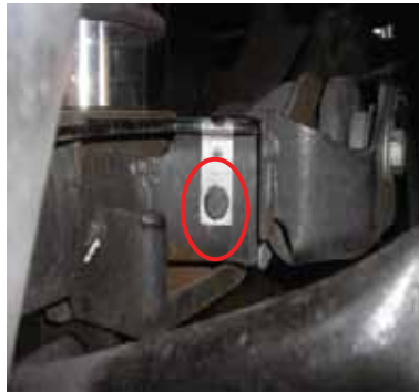
2. Unhook the ABS line at the frame on the both sides.
