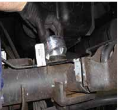
7. Remove the 13mm emergency brake line support bracket on the passenger side frame rail.
