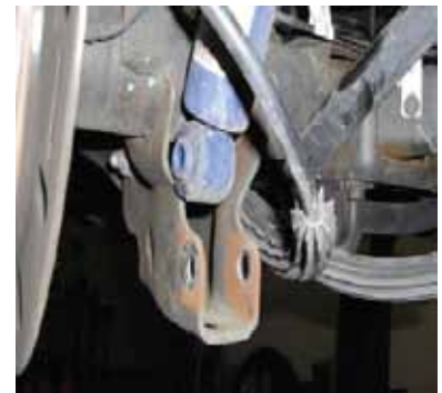
6. Unbolt the passenger side hard brake line support bracket bolt.
